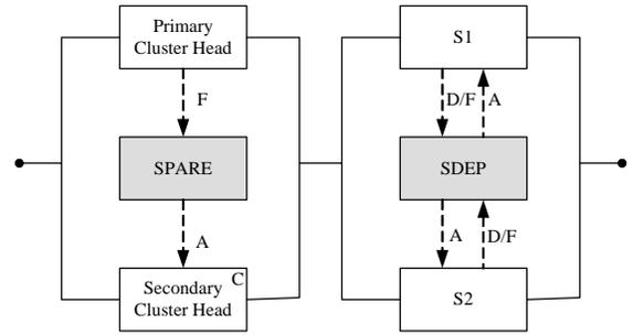
**Figure 4.** The DRBD model of the example system
