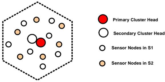
**Figure 1.** A clustered wireless sensor network system
