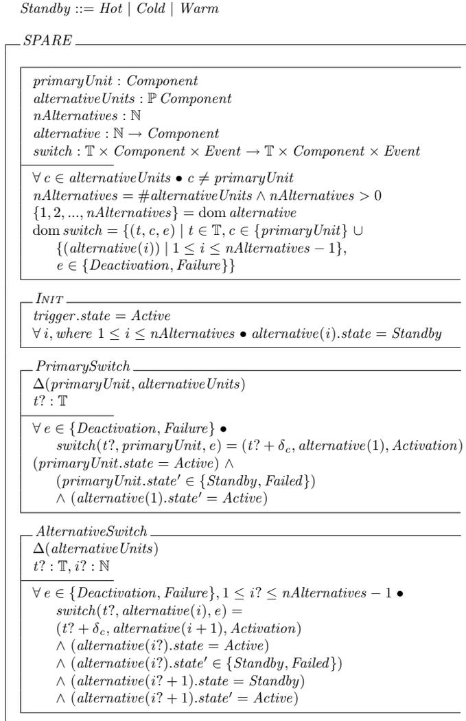
Fig. 8. Object-Z Specification of SPARE Block
