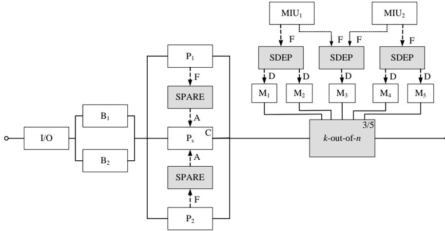
Fig. 4. The DRBD Model of the HECS
