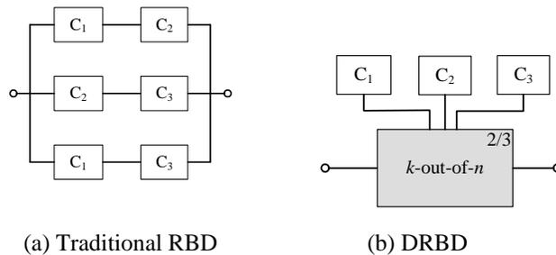
Fig. 3. Representation of a 2-out-of-3 Structure
