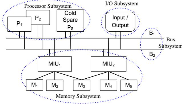
Fig. 1. An Example Computer System (Adapted From [5, 6])
