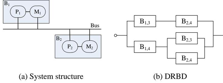
Fig. 5. Example Multistate System and DRBD Model
