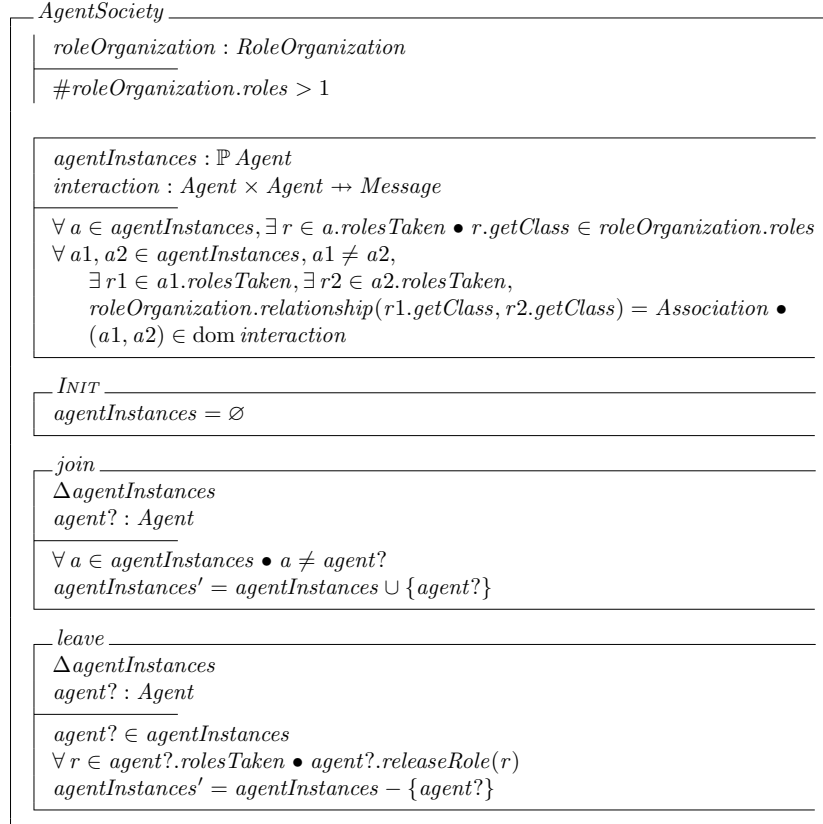
Figure 6. Formal specification of the AgentSociety class in Object-Z
