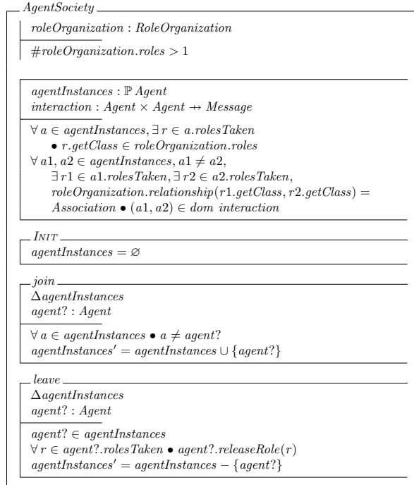
Figure 6. Formal Specification of the AgentSociety Class in Object-Z
