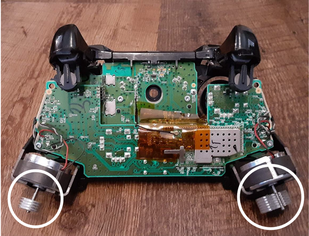
Fig. 5. The internal hardware of an Xbox controller with two different vibration motors circled [12]. The left motor's weight is much larger than the right motor's weight (the controller is face-down in this image). This image is licensed under the Creative Commons Attribution-Share Alike 4.0 International license and was modified by the author to draw attention to the motors.
