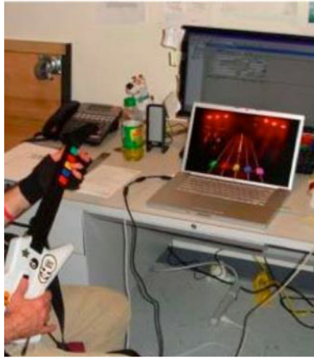
Fig. 6. A blind user wearing the custom haptic glove created for Blind Hero to play using a Guitar Hero guitar controller [15]. This image has been modified by the author to remove identifying features of the player.
