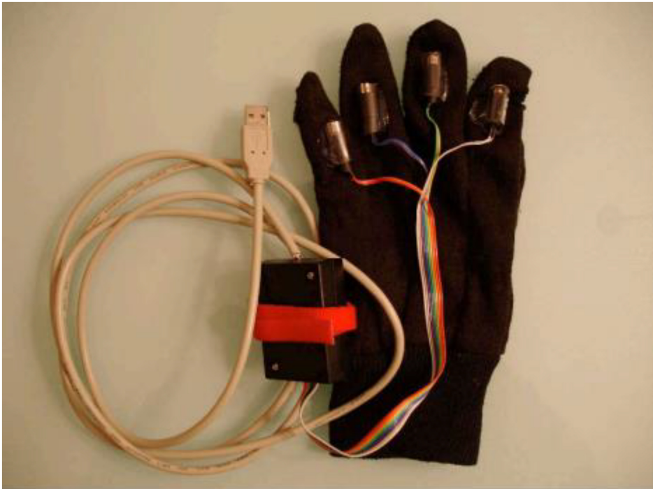
Fig. 7. The haptic glove controller that was custom engineered for Blind Hero. At the time, this device cost around $1,500 total to develop and allowed the user to feel incoming notes on each fingertip with the use of haptic motors [15].
